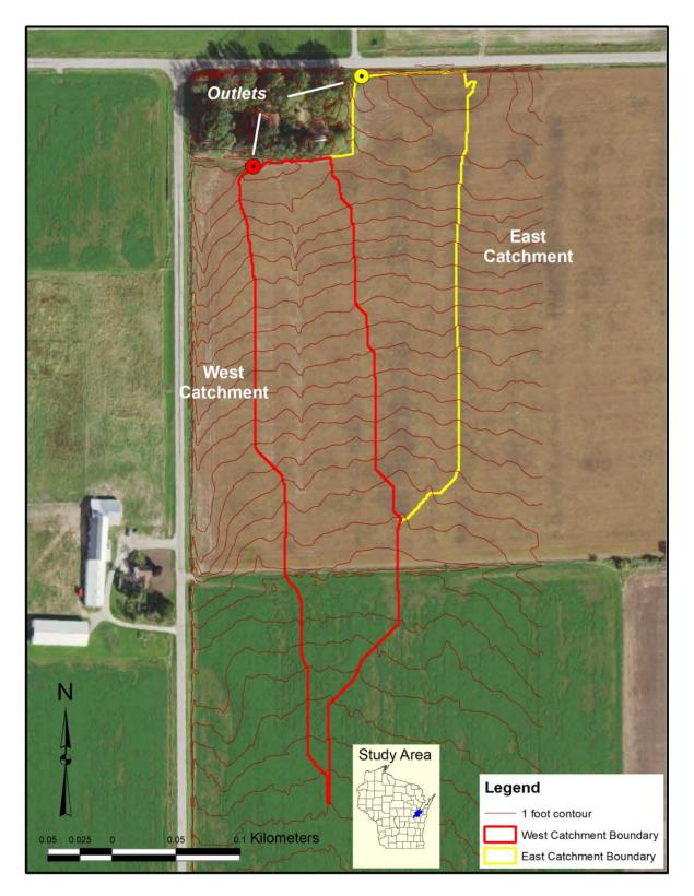
Figure 2. Study site with 1 foot elevation contours and east and west catchment boundaries and outlets to edge-of-field monitoring stations. Contour shapefile based on 2018 LIDAR was obtained from the Calumet County Land Information Office. Background is USDA FSA aerial orthophoto from 2017.
