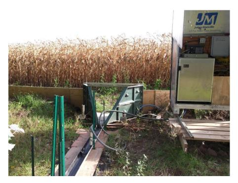
Figure 3. Station housing and monitoring equipment at outlet of west catchment. Turbidity probe is mounted below flume in half-pipe.
